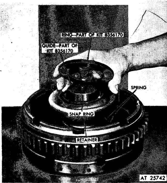
Figure 5-70. Positioning snap ring and replacer components on high-range clutch assembly using ring and guide (part of kit 5180-572-8607 (8356170)).
